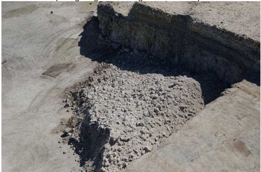
Figure 2: 3D image of the blast pile used for fragmentation analysis
