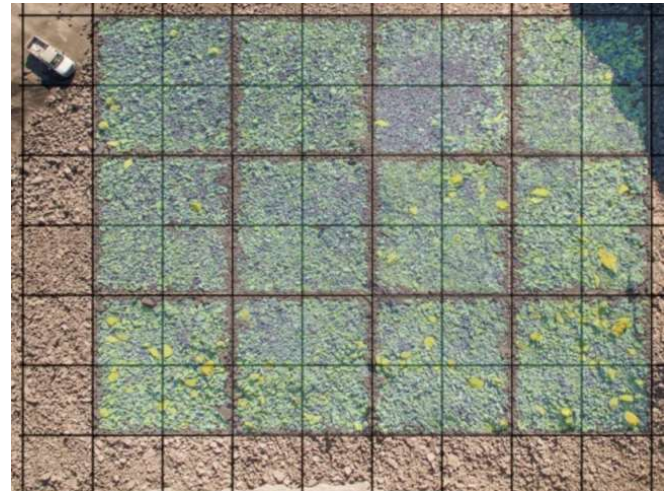
Figure 10: Fragmentation grids can be colour coated based on sizes, and can identify areas in the pit that showed finer and coarser fragmentation
